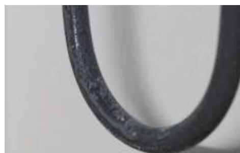
Heater with defective protective coating!
